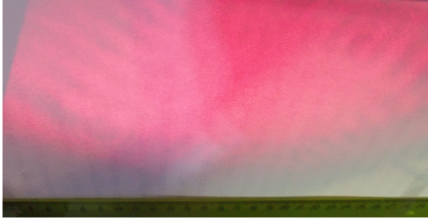
Figure 2: Projection image of the transverse structure of a low-quality semiconductor laser beam obtained with a projection magnification of approximately M = 300 . The image reveals pronounced spatial inhomogeneity, concentric interference rings, and fine layered intensity modulation that are essentially invisible under ordinary observation conditions.
