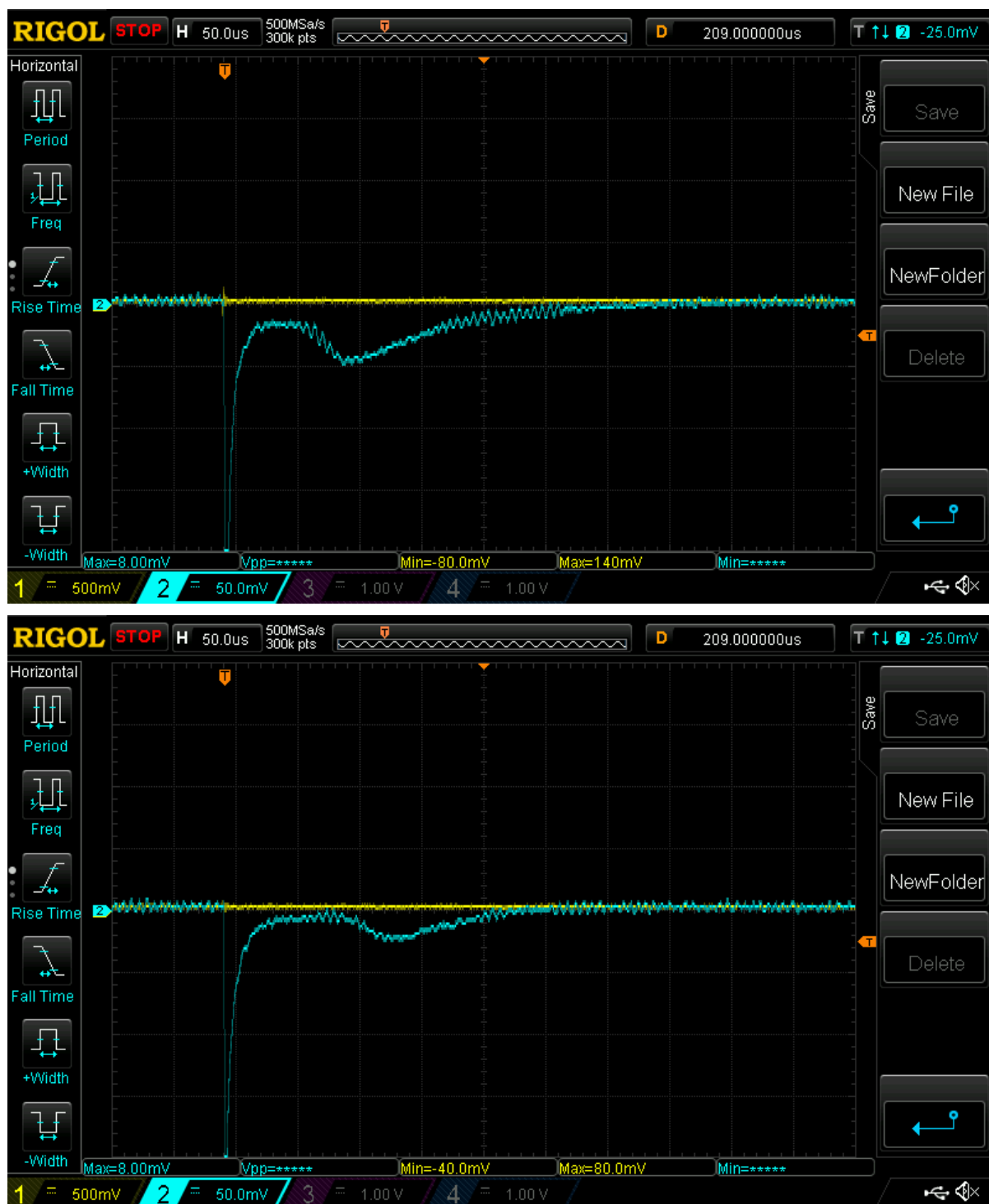
Fig. 21. Signal from microwave sensor from two different shots. Charging voltage of first PFL 400 kV. Air, 0,5 mbar. 11 mm hole diode.
