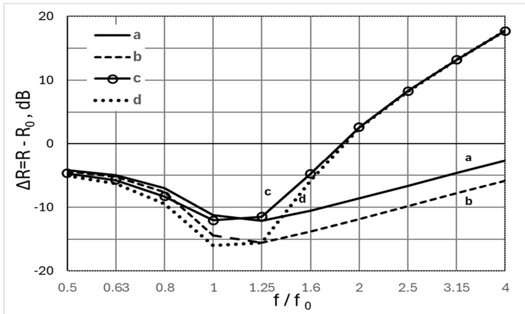
Figure 5: Relative frequency characteristics  $\Delta R$ , calculated at  $\theta_m = 90^\circ$  for the single-space model with air and krypton fills: a – air,  $\eta_c=0.2$ ; b – air,  $\eta_c=0,1$ ; c – krypton,  $\eta_c=0.28$ ; d – krypton,  $\eta_c=0,14$ .
