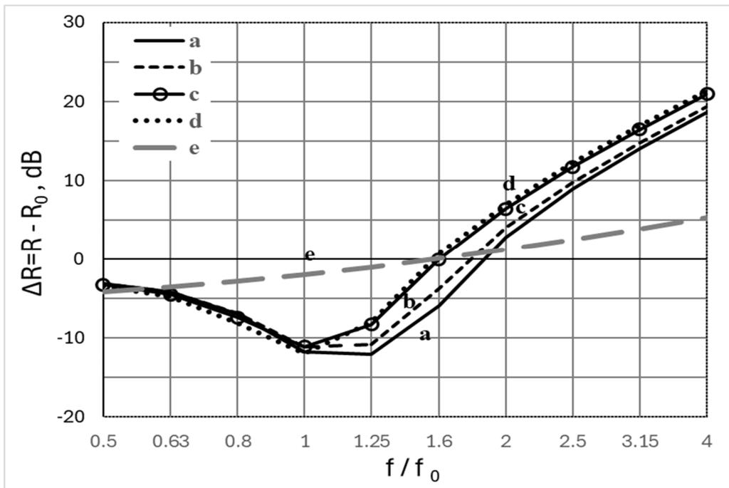
Figure 6: Relative frequency characteristics  $\Delta R$ , calculated for flanking sound transmission (e) and direct transmission at  $\theta_m = 45^\circ$  via the single-space model with air (a), argon (b), krypton (c), and xenon (d) fills.
