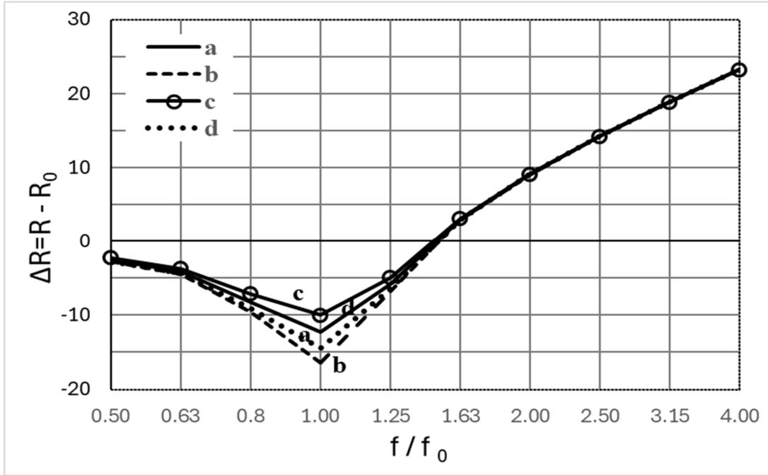
Figure 2: Relative frequency characteristics  $\Delta R$ , calculated at  $\theta_m \rightarrow 0^\circ$  for the single-space model with air and krypton fills: a – air,  $\eta_c=0.2$ ; b – air,  $\eta_c=0.1$ ; c – krypton,  $\eta_c=0.28$ ; d – krypton,  $\eta_c=0.14$ .
