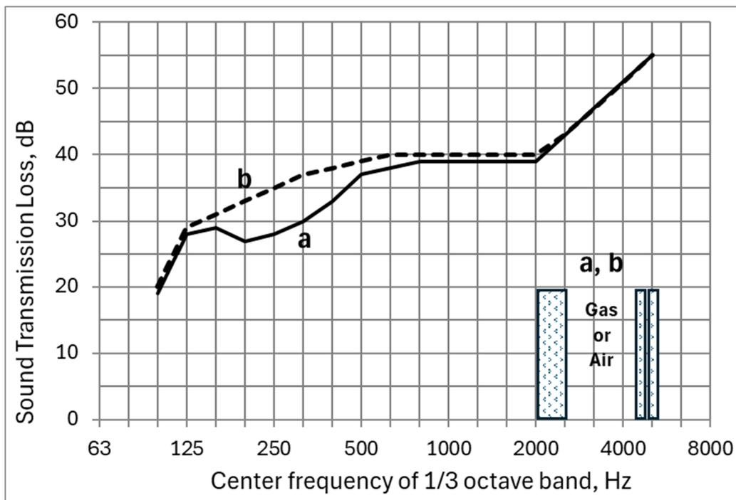
Figure 9: Frequency characteristics of sound transmission loss measured for double-space IGU (10+20+5+0.5+6): a – filled with air, b – filled with gas mixture, 73% Freon-12, 27% air.
