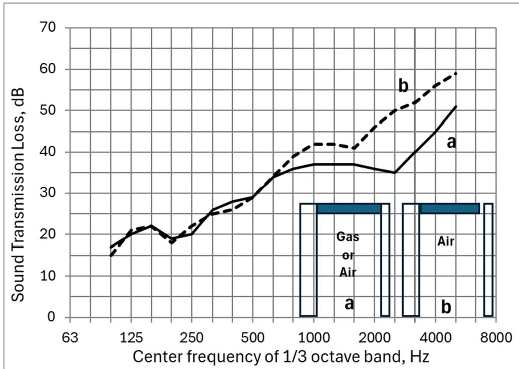
Figure 8: Frequency characteristics of sound transmission loss measured for single-space IGU (8+12+5): a -original specimen, b –the structural links between the panes are weakened.
