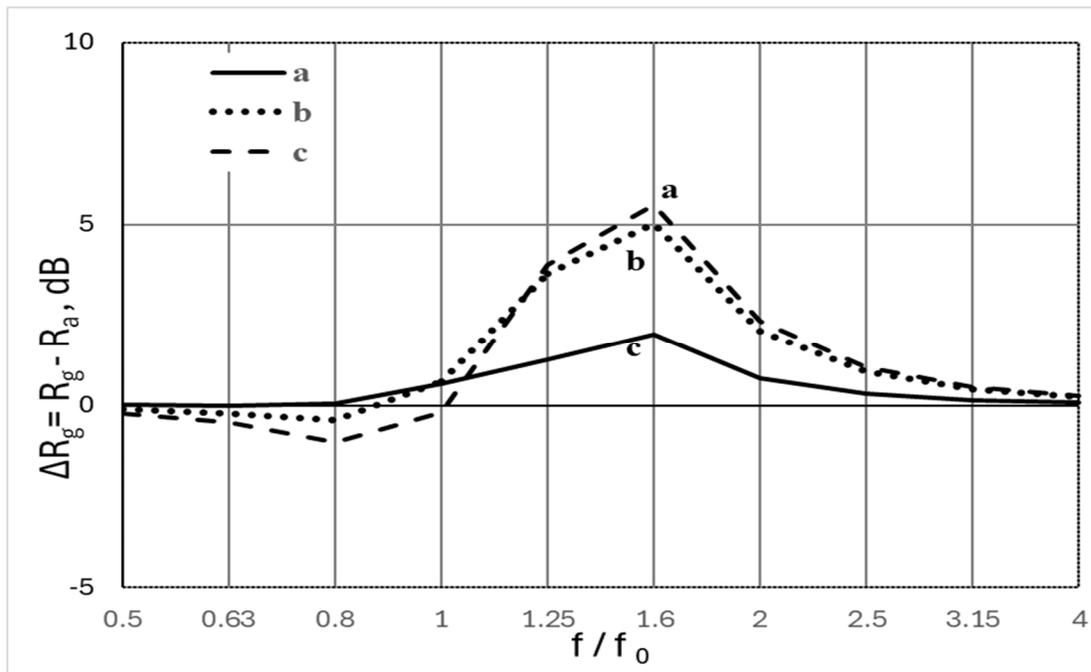
Figure 7: Calculated increase in sound transmission loss for single-space IGU filled with (a) xenon, (b) krypton, and (c) argon compared to that for the same IGU filled with air. Here,  $\theta_m = 45^\circ$ .
