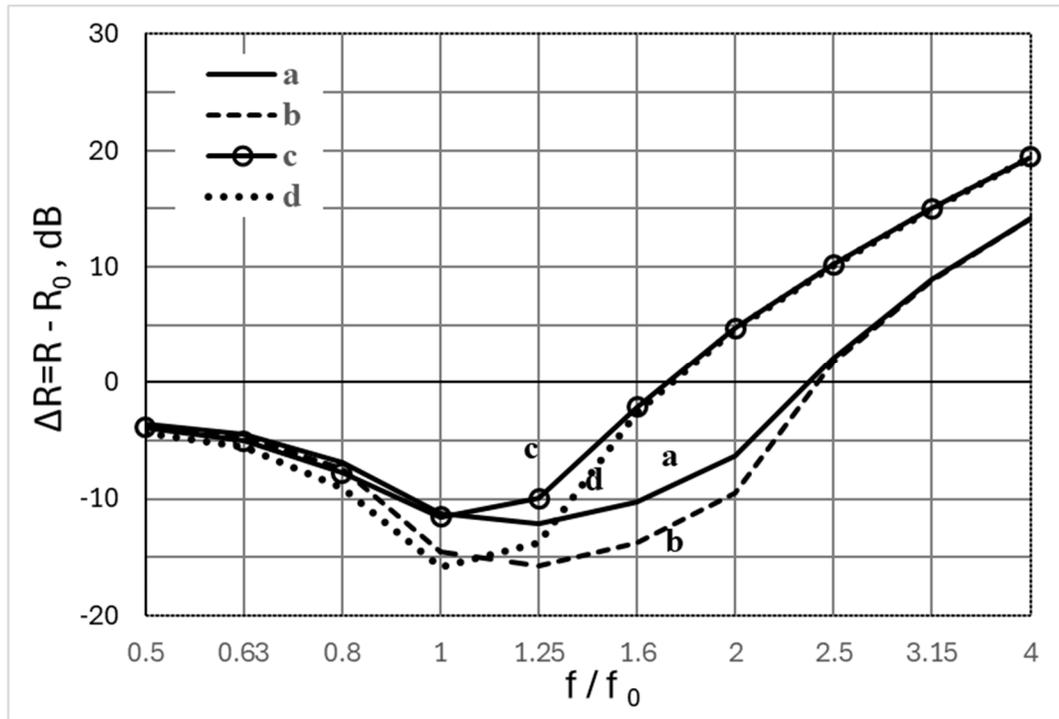
Figure 4: Relative frequency characteristics  $\Delta R$ , calculated at  $\theta_m = 60^\circ$  for the single-space model with air and krypton fills: a – air,  $\eta_c=0.2$ ; b – air,  $\eta_c=0,1$ ; c – krypton,  $\eta_c=0.28$ ; d – krypton,  $\eta_c=0,14$ .
