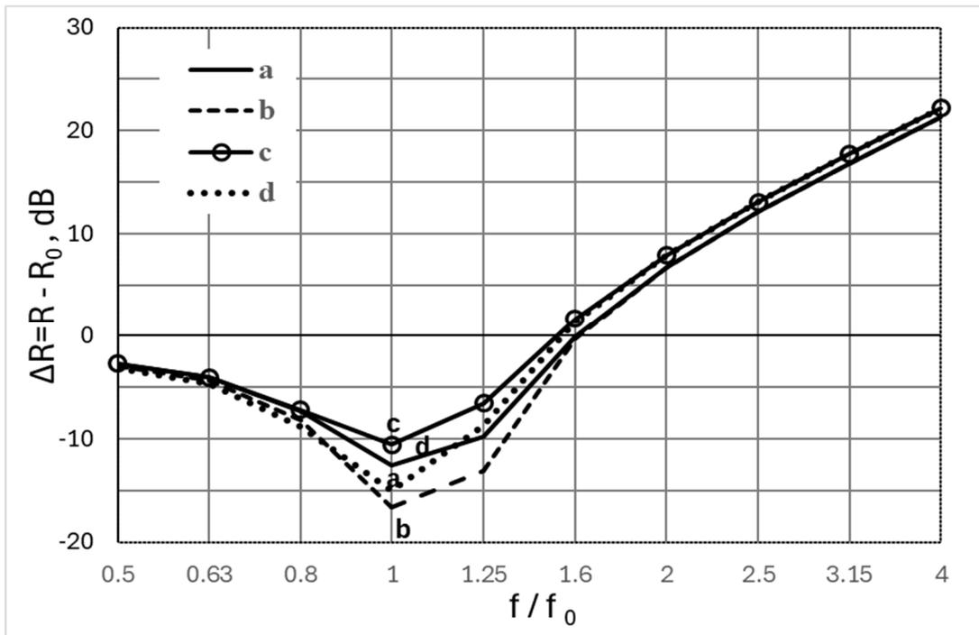
Figure 3: Relative frequency characteristics  $\Delta R$ , calculated at  $\theta_m = 30^\circ$  for the single-space model with air and krypton fills: a – air,  $\eta_c=0.2$ ; b – air,  $\eta_c=0.1$ ; c – krypton,  $\eta_c=0.28$ ; d – krypton,  $\eta_c=0.14$ .
