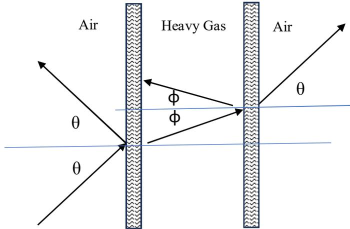
Figure 1: Direct sound transmission via gas-filled double glazing at oblique incidence.
