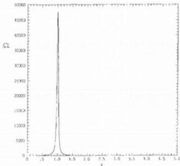
Fig. 2. Cross section of vorticity distribution in 80-vorton ring.
