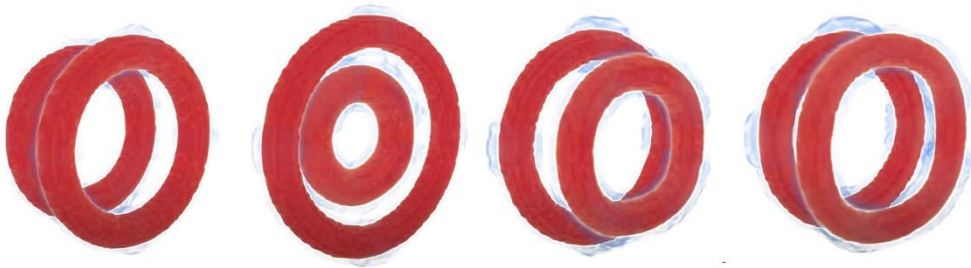
Figure 1 shows a section of the continuous looping exhibited by ring vortices
