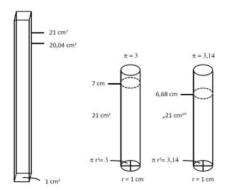
The well-known definition of 1 cm<sup>3</sup> (1 ml) is a cube with a side length of one. Fig. 2 shows a box-shaped container with a bottom area of exactly 1 cm<sup>2</sup>. Therefore; any length of the container corresponds exactly to the amount of cm<sup>3</sup> (ml) to the amount in cm<sup>3</sup> (ml) of e.g. of a liquid contained therein:
