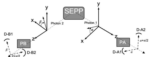
Figure 1: The SEPP (source of entangled photon pairs) emits entangled photons propagating towards the adjustable polarizers PA and PB and detectors DA-1 and DA-2 on wing A and DB-1 and DB-2 on wing B. A coincidence measuring device (not seen in the picture) encounters matching events. The
