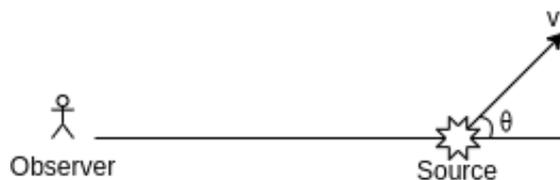
Figure 8: Doppler shift for a moving source
