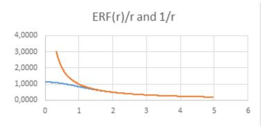
Due to the convolution, and the coherence of the location density distribution, the blue curve does not show any sign of the singularity that is contained in the red curve, which shows the Green's function.
