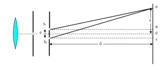
FIG. 1. Double Slit Interference
