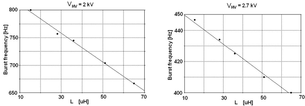
**Fig. 2.** Burst rate dependence on external inductance  $L_I$  for 2 kV and 2.7kV. Vacuum cell with air at 11 mbars.
