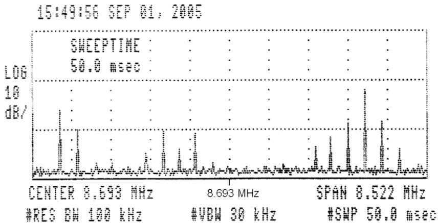
Fig. 14. Hydrogen spectrum, 50 ms sweep time [6]
