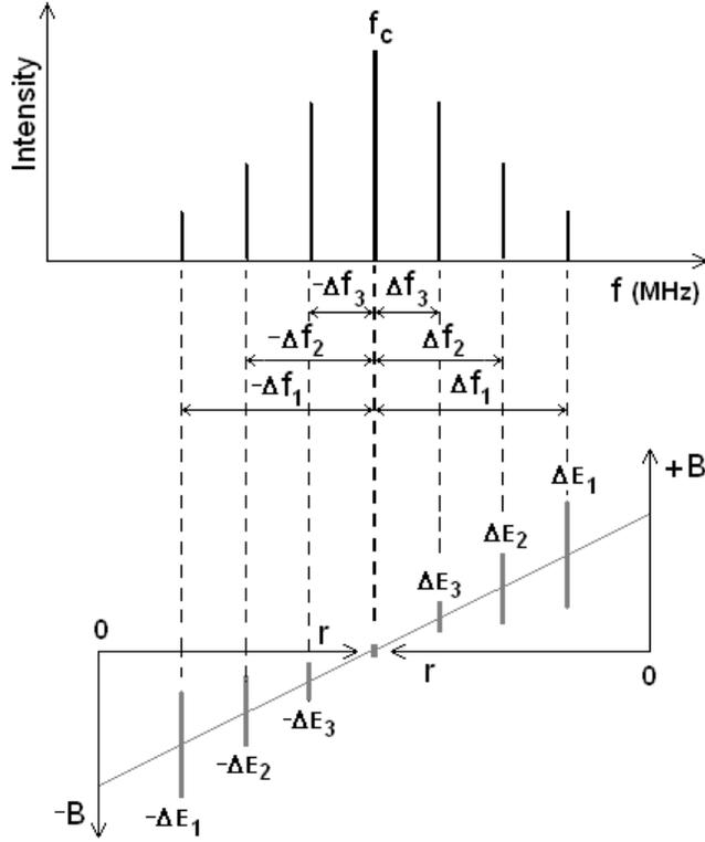
**Fig. 10.** Graphical illustration of the physical parameters behind the observed frequency spectrum due to electron spin flip. The upper coordinates are in the frequency domain, while bottom coordinates  $+B$  and  $-B$  are shown as a function of  $r$ , but  $r$  for  $+B$  and  $-B$  are shown in opposite direction in order to match the spectrum domain.
