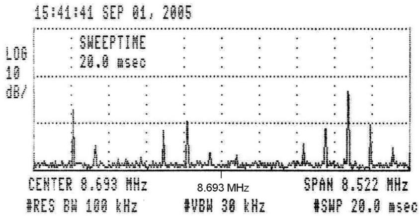
Fig. 12. Hydrogen spectrum, 20 ms sweep time [6]
