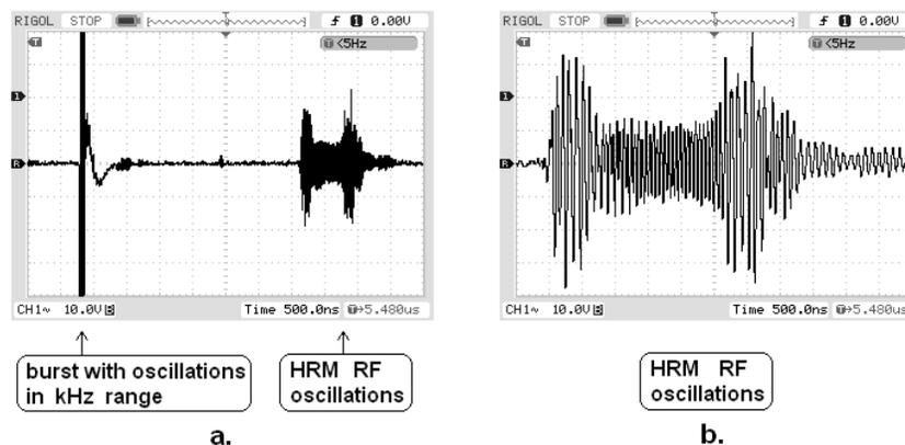
**Fig. 1.** Waveforms of glow discharge of air at 11.5 mbars, a. – burst rate with the HRM oscillations, b. expanded view of the HRM oscillations
