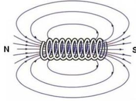
**Fig. 9.** Magnetic field of the single layer solenoid.
