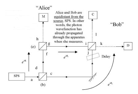
Figure 4 – Ports of the 1-photon device enumerated
