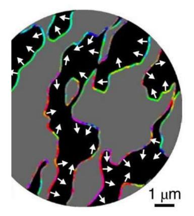
In these images developed using the SPLEEM instrument at Berkeley Lab, the orientation of magnetization in samples containing cobalt (Co) and ruthenium (Ru) is represented with white arrows. The image at left shows how the orientation is ...<u>more</u>
