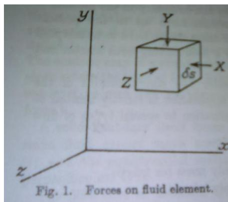
Fig. 1 – Forces on fluid element.
