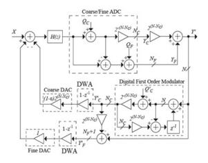
Figure 6: Mathamatical Block Diagram of ReQ Metode.
