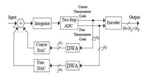
Figure 2: Block Diagram of Segmentated  $\sum \Delta$  ADC.
