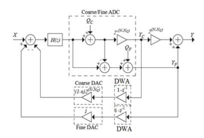
Figure 3: Mathematical Block Diagram of Segmented  $\sum \Delta$  ADC.
