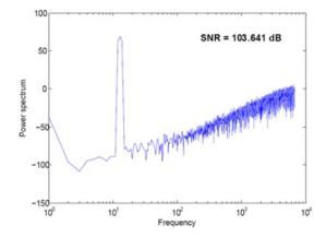
Figure 7: Output Spectrum the  $\sum \Delta$  modulator using method requantization.
