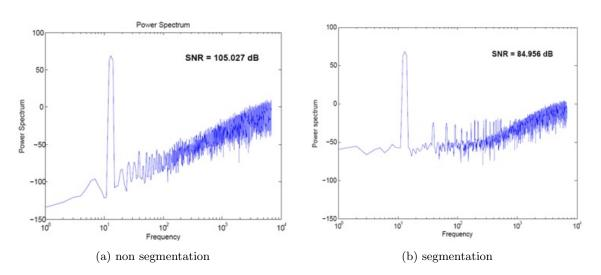
Figure 4: Output spectrum of the  $\sum \Delta$  modulator employing (a)non segmentation and (b)segmentation.
