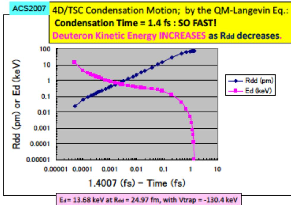
... The ‘adiabatic’ size of 4D/TSC reaches at a few tens fm size in 1.4 fs, so fast. With adiabatic 4D/TSC size around 20 fm, 4D-fusion takes place by ...
