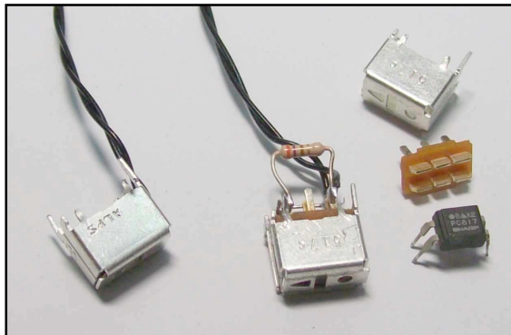
Fig. 1 : g-sensor (left) and assembled photocoupler (mid) with his parts (right)
