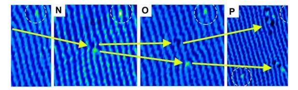
Cooling sample. The yellow arrows indicate the vortex-antivortex pair, as it is generated (N), separates (O), and further diverges (P). The authors note that the process is observed at domain junctions called Y dislocations (as in M) or on ...more
