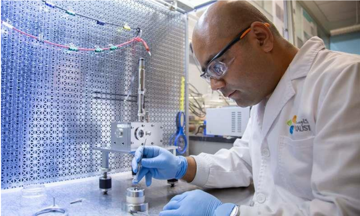
Buddha Shreshtha loads a silica disk with an ultrasmooth-surface terminated with per fluorocarbons comprising 10 carbon atoms. Credit: © 2019 KAUST
