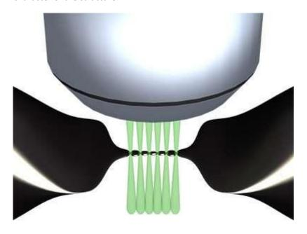
Atoms are shaped into a wire using laser light. Their flow can be influenced by projecting a variable number of light obstacles focussed on the wire with a microscope objective. Credit: Esslinger group/ETH Zurich
