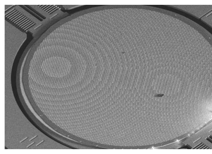
In this image, a circular metasurface-based flat lens has been integrated onto a MEMS scanner. Integration of MEMS devices with metalenses combine the strength of high-speed dynamic control with precise spatial manipulation of wave-fronts. ...more
