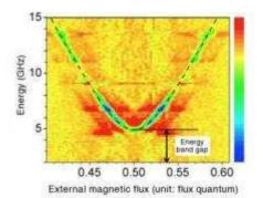
An energy band gap is obtained using energy spectroscopy. Existence of band gap establishes that coherent tunneling has occurred. Credit: RIKEN
