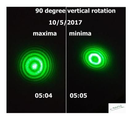
For more than 90° rotation I have a positive chnge in the central interference pattern from maxima to minima to maxima in the central interference pattern
