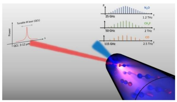
Artistic view of the QCL pumped terahertz laser showing the QCL beam (red) and the terahertz beam (blue) along with rotating molecules inside the cavity. The figure shows emission spectra of each gas.
