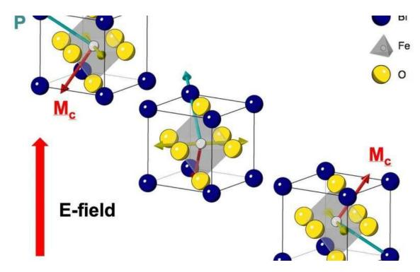
Single crystals of the multiferroic material bismuth-iron-oxide. The bismuth atoms (blue) form a cubic lattice with oxygen atoms (yellow) at each face of the cube and an iron atom (gray) near the center. The somewhat off-center iron ...<u>more</u>Internet of things and AI
