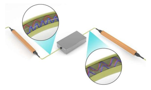
The researchers' innovative experimental setup involved operating on photons contained within a single fiber-optic cable. This provided stability and control for operations producing entangled photons, shown separated at top and intertwined ...<u>more</u>"We were able to extract more
