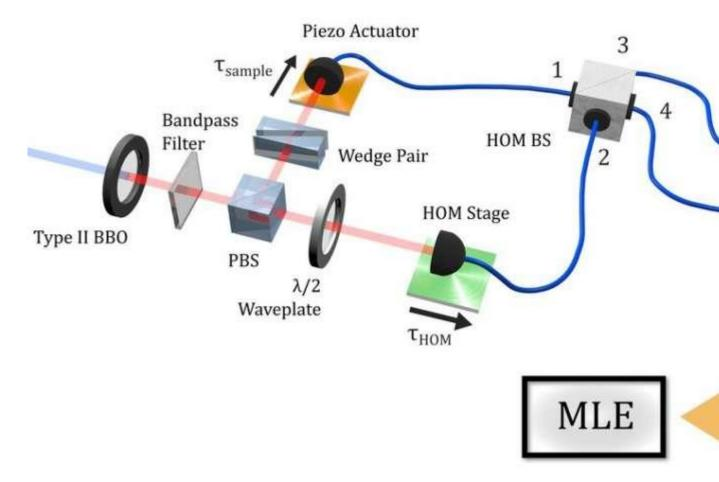
Diagram showing the technique for measuring nanoscopic structures. Credit: University of Warwick
