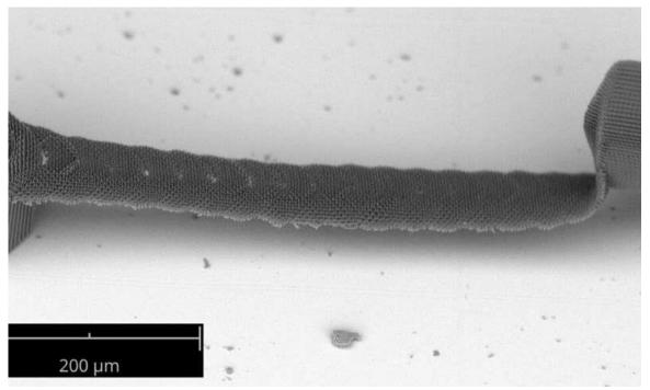
Overhanging 3D structures printed by stitching multiple 2D projections, demonstrating the ability to print depth-resolved features. The bridge structure, with 90-degree overhangs, is challenging to print using serial scanning TPL techniques. Credit: Vu Nguyen and Sourabh Saha
