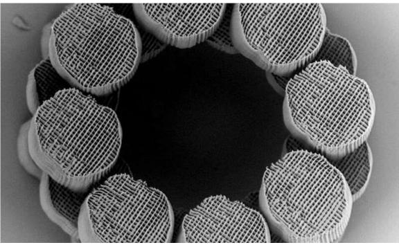
A stacked 3D ring structure generated by overlapping several projections in 3D space. Arbitrarily complex 3D structures can be generated through this depth-resolved nanoscale 3D printing technique. Credit: Vu Nguyen and Sourabh Saha
