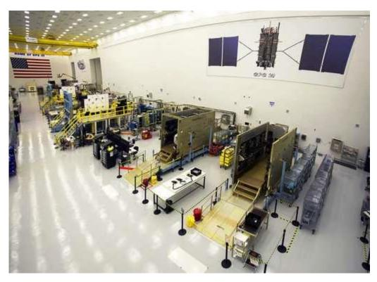
This Sept. 2, 2016 photo provided by Lockheed Martin shows GPS III satellites being built in a clean room at Lockheed Martin's complex south of Denver. The first GPS III satellite is scheduled to be launched from Cape Canaveral, Fla., on ...more
