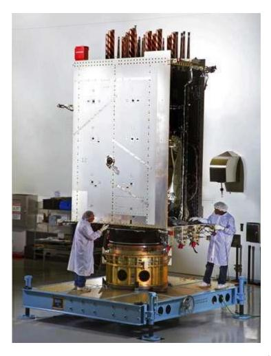
This April 9, 2015 photo provided by Lockheed Martin shows the first GPS III satellite being built in a clean room at Lockheed Martin's complex south of Denver. The satellite is scheduled to be launched from Cape Canaveral, Fla., on ...more
