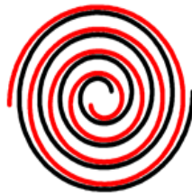
clockwise and anticlockwise winding
