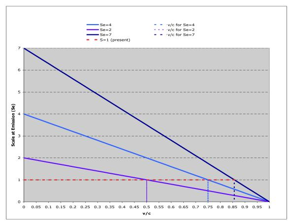
**Fig 4** Illustration of  $S_e = 1/(1-v/c)$
