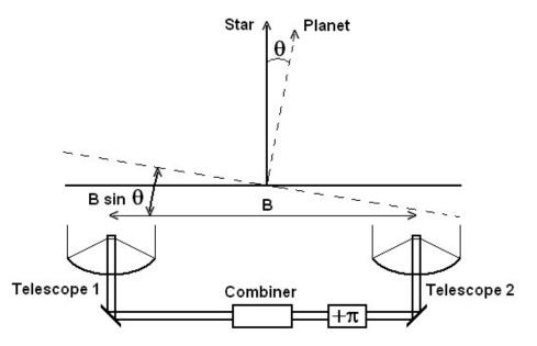
**Figure 1**. Two telescope space-based nulling interferometer, simplest config-uration for producing a dark fringe in the line of sight when properly phased. This destructive interference enables planet detection by subtracting stellar coronas when focusing the null region on the stars disk. Redrawn from [63].
