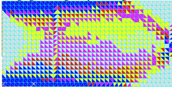
Fig. 7. checkerboard pattern.
