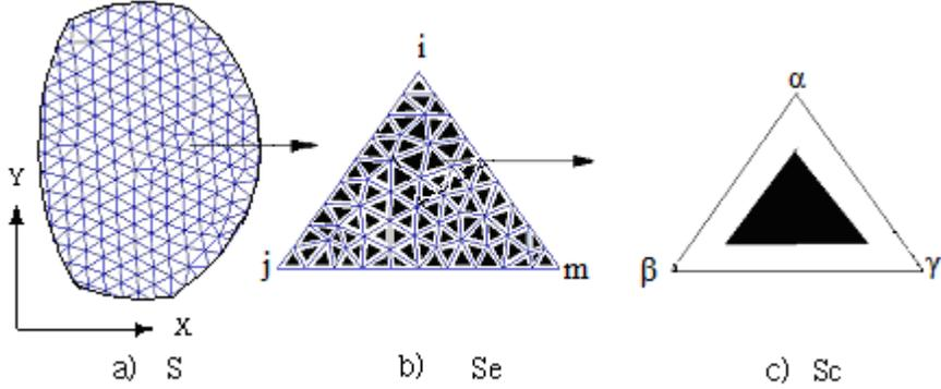
Fig. 1. Geometry model (a) design domain, b) element, c) cell)
