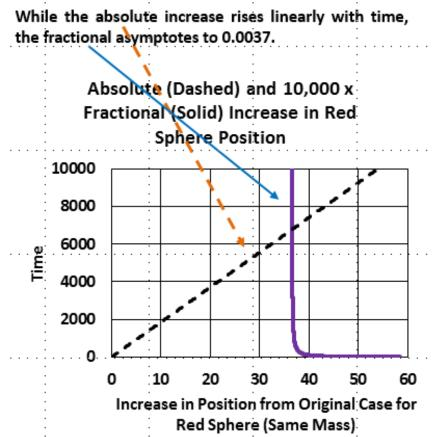
Figure 7. Case 3 - Absolute and 10,000 x Fractional (Solid) Increase in Red Sphere Position
