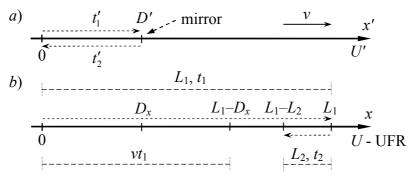
Fig. 2. The light flow time and path to the mirror and back: (a) the way of light seen from the inertial system U', (b) the way of light seen from the ether.
