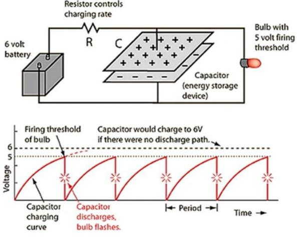
FIGURE 3. Circuit Schematic for a Strobe Device
