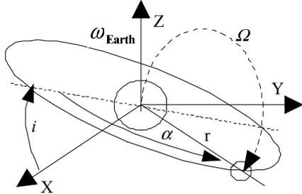
Fig. 2.2 : Definition of the angles  $\alpha$  and  $i$ . The orbital plane is defined by the orbital inclination  $i$  in relation to the axis  $X$ . The location of the satellite inside the orbit is defined by the angle  $\alpha$ . The equipotential line of the gyrotation  $\Omega$  through the satellite has been shown as well.
