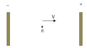
Suppose that the electron is initially moving with some constant velocity V. This can be done by initially switching on the voltage across the plates briefly and switching it off, discharging the plates so that the electric field will be zero. With zero electric field, the electron will continue moving with a constant velocity.
