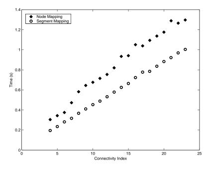
Figure 6: Execution time in seconds versus the average connectivity index of the network for the node mapping and segment mapping algorithms. All networks used in these tests have a single section with five million nodes.
