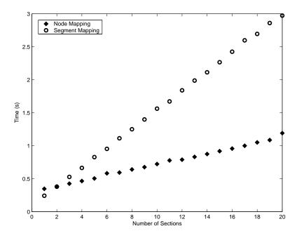
Figure 7: Execution time in seconds versus the number of network sections for the node mapping and segment mapping algorithms. All networks used in these tests have about five million nodes with an average connectivity index of approximately 5.
