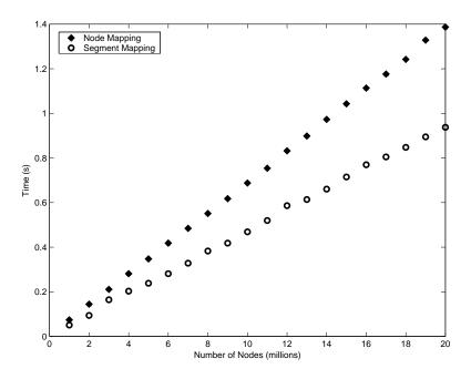
Figure 5: Execution time in seconds versus the number of network nodes in millions for the node mapping and segment mapping algorithms. All networks used in these tests have a single section with an average connectivity index of approximately 5.
