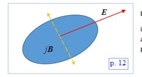
Vector E belongs to the plane defined by bivector jB. Area of the circle which presents bivector is B, so its radius must be  $\sqrt{B/\pi} \approx 0.56\sqrt{B}$ . Direction and possible orientations of wave propagation are plotted in p. 12.
