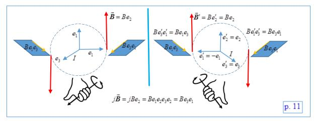
multiplying it by a complex phase, like  $e^{j\omega t}$ , so, we have a spiral in space which rotates around the direction of propagation of the wave. Bivector part jB defines the plane orthogonal to B, so vector E belongs to that plane. Bivector jB provides an opportunity for consideration of electromagnetic phenomena more complete and more elegant than (axial) vector B.
