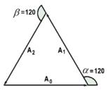
Fig. 2 Phasor diagram of three waves in perfect destructive interference.
