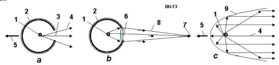
**Fig.7.** AB- Generator as Photon Rocket and Radiation (Photon) Weapon. (a) AB- Generator as a Simplest Photon Rocket; (b) AB- Generator as focused Radiation (photon, light or laser) weapon; (c) Photon Rocket with Micro-Black Hole of AB-Generator. *Notations*: 1 – control MBH; 2 – spherical cover of AB-Generator; 3 – window in spherical cover; 4 – radiation of BH; 5 – thrust; 6 – lens in window of cover; 7 – aim; 8 - focused radiation; 9 – parabolic reflector.
