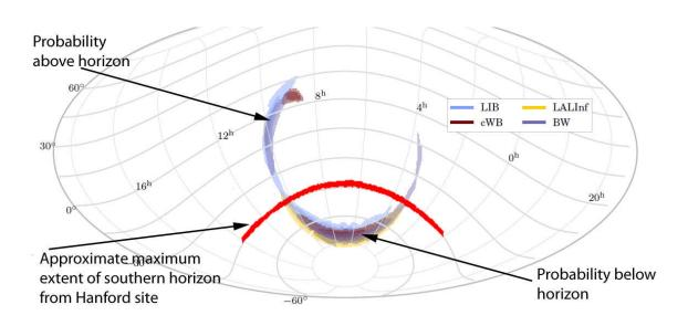
Fig 1. All-sky projections of in celestial coordinates showing probability of source location by the use of burst algorithms. [12] The diameter of the annular circle is defined by the 6.9 ms separation of the signal from the two sites. The distributed probability is defined by analysis using 4 different burst algorithm analyses of the signals. The red line is the maximum southern extent that the event could be located and still have line of sight visible from Hanford. (Appox. -  $44^{0}$ )
