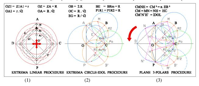
F.48. The three Circles, [Inscribed – Circle – Circumscribed ], on any diameter OB of a Circle, The common Radical axis of the system and Euler-Savary Plane Kinematic of Mechanics.
