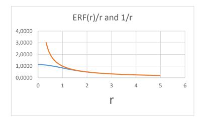
We suppose that this distribution is a good estimate for the structure of the swarm of a free electron. It is remarkable that this potential (the blue curve) has no singularity at R=0. At the same time, already at a short distance of the center the function very closely approaches 1/R (the orange curve).
