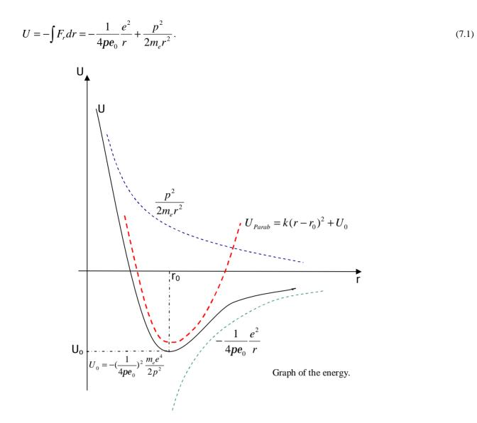
The point of minimum in  $(r_0, U_0)$  is a balance and stability point  $(F_r=0)$  and can be calculated by zeroing the first derivative of (7.1) (i.e. setting  $F_r=0$  indeed).
