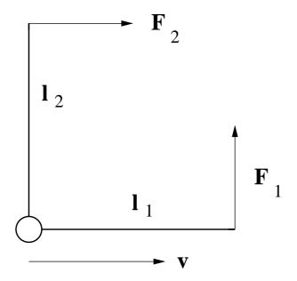
Figure 4.10: Paradox of a lever.
