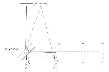
Figure 3.2: Scheme of the interferometer.
