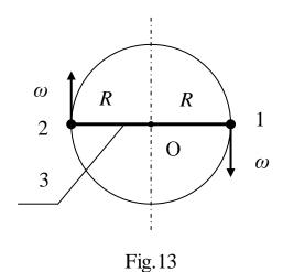
Bodies 1 and 2 are connected by a string 3, the mass of which can be neglected because of its smallness.
