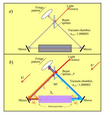
Fig 2. The optical scheme of forming beams of the interferometer, proposed by the authors [1]: a) the expected by the authors [1] idealized scheme of the course of optical processes in the unusual onerod interferometer-detector of "aether wind";
