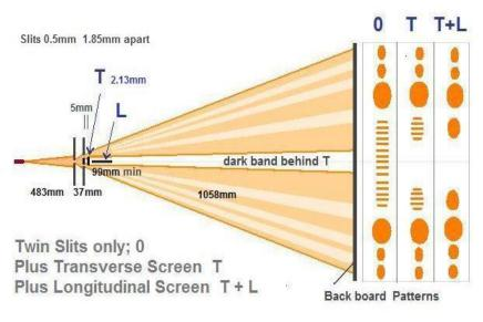
Overlapping light paths blocked by transvers screen T. 5mm behind twin slits (with edges in dark bands) Part of interference pattern remains. When lateral screen L is introduced in the dark band behind T the remaining interference pattern is lost.
