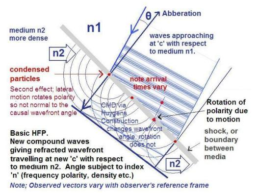
**Figure 8.** Huygens Fresnel Principle HFP Refraction. (extended). Common refraction is towards the normal (perpendicular) to the refractive plane. For media in relative motion light speed is converted to the new local 'c' (or c/n) and varies subject to the observers frame. In the DFM two related effects are combined; Chromatic Mode Dispersal (CMD) due to propagation speed change, and polarity rotation due to co-motion on charging.
