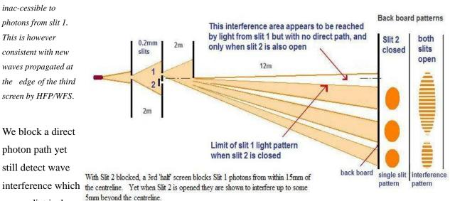
*Figure 10b.* Double Slit Variation b. A third screen edge is positioned on the centreline. Interfer-ence still occurs in the central zone inac-cessible to
