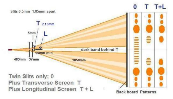
Overlapping light paths blocked by transvers screen T. 5mm behind twin slits (with edges in dark bands) Part of interference pattern remains. When lateral screen L is introduced in the dark band behind T the remaining interference pattern is lost.
