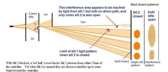
*Figure 10b. Double Slit Variation b.* A third screen edge is positioned on the centreline. Interference still occurs in the central area inaccessible to photons from slit 1 without an exceptional refraction angle. This is however consistent with new oscillators or waves propagated at the edge of the third screen by HFP and WFS. (Fleagle 'Separated Pattern').
