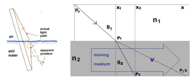
*Fig 1. Refraction.* Between different media such as air and water actual refraction is inverse to apparent path change observed from each medium. For media in relative motion (even of similar refractive index) the same applies. Here the observer *changes inertial frame* with the 'ray' of light. Lodge showed the 'ray' following the red path. Viewed from frame  $n_2$  it actually refracts in the opposite direction, to  $P_2$
