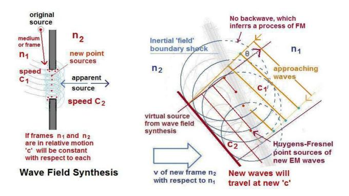
*Figure 7.* Huygens-Fresnel Principle, Fourier Optics and Wave Field Synthesis deriving a virtual source, inferring that waves from new point sources in new frames will travel at 'c' with respect to the new frame. Note the new wavelength has changed with vector, conserving frequency and energy.
